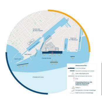
Eole infrastructures: Assembly Quay Float Storage Area Onshore Storage Area Service Vessel Pontoon Crane Components present on site during floating wind turbine assembly operations: Floats Components awaiting assembly
